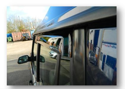
Rear deflectors should align perfectly with the door frame.
