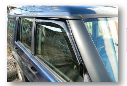
Ensure the right angle on the deflector meets the right angle of the mirror mounting.
